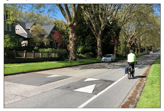
Figure 5 – Raised crosswalk (North Vancouver BC)
