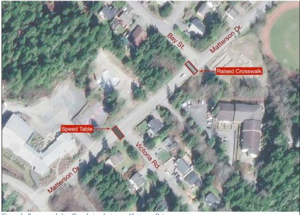
Figure 1– Recommended traffic calming devices on Matterson Drive
